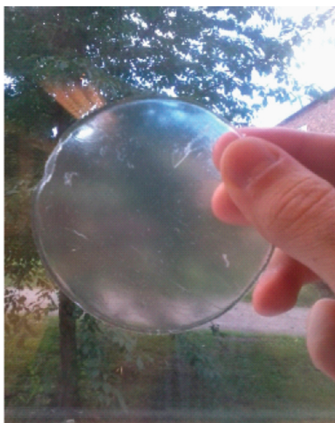
Figure 3. TEMPO-NFC cake obtained after vacuum filtration of TEMPO-NFC aqueous dispersion (water content in the cake is 70–90%).
